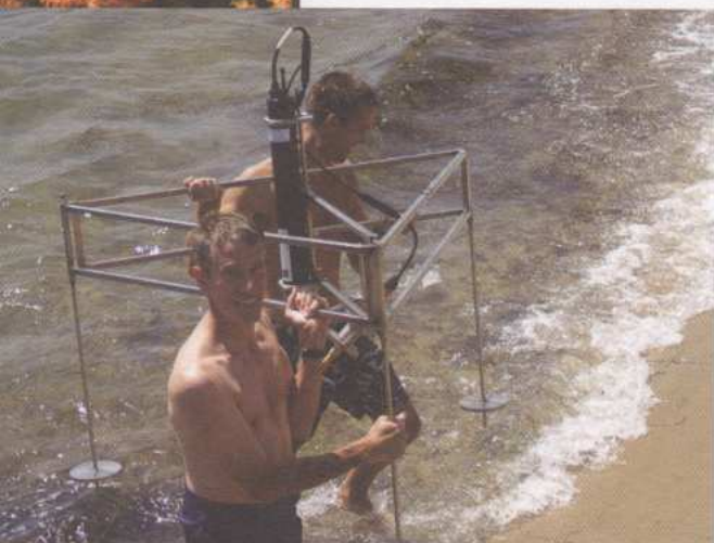
Peter Berg (left) worked with colleagues in Germany to apply eddy correlation techniques underwater.
